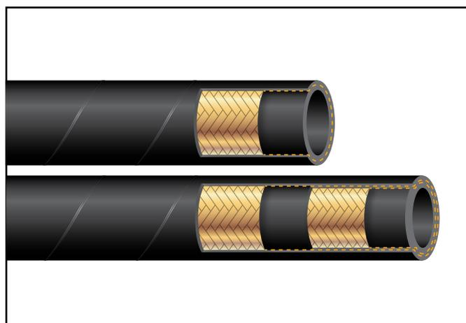
**APPLICATIONS:** Used for medium pressure hydraulic lines on mobile equipment, machine tools and farm equipment. Meets or exceeds SAE 100R17.
