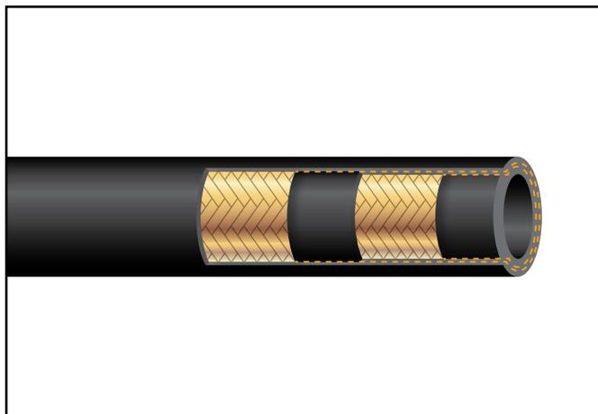
**APPLICATIONS:** Used for high pressure hydraulic lines on off-road construction equipment, machine tools and farm equipment. Meets or exceeds SAE 100R16 (Type 2SC).
