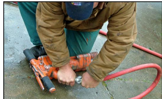
**CONSTRUCTION:** EPDM tube, red EPDM cover, reinforcement is multiple spiral polyester yarn
