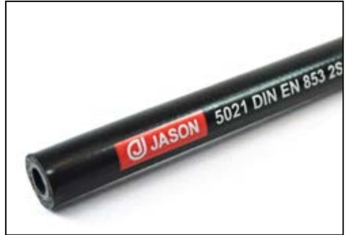
**APPLICATIONS:** Used for high pressure hydraulic lines on off-road construction equipment, machine tools, farm and marine equipment. Meets or exceeds SAE 100R2 and EN 853 2SN.
